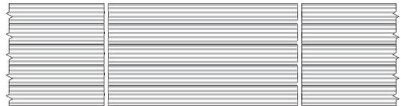
Reveals (1”) can be **Symmetrical** giving a linear appearance or **Staggered** to minimize joint layout
